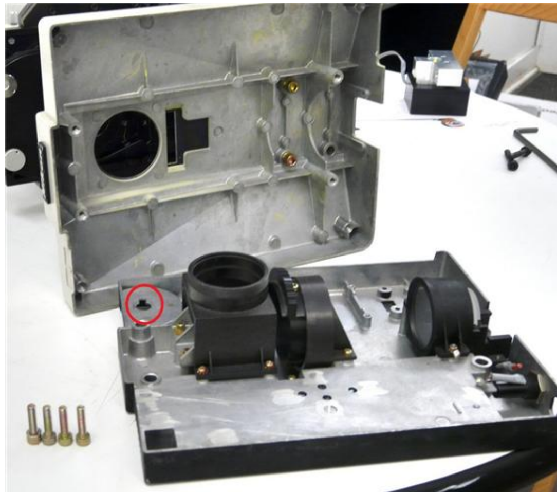
(2) Bottom cover removed. Note that the pot will still be in place at the red circle, and the electronics were stripped out before we got it.
