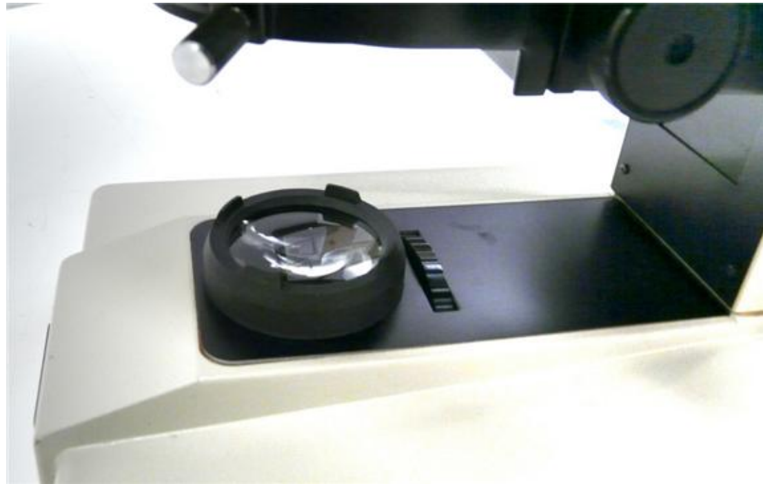
(1) The black ring around the lens must be removed to open the microscope.
