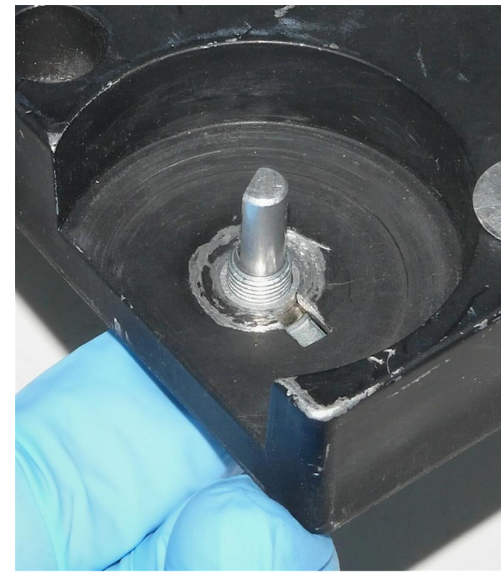
(3) Install the Nanodyne pot as shown. Be sure the metal centering bushing is in place.
