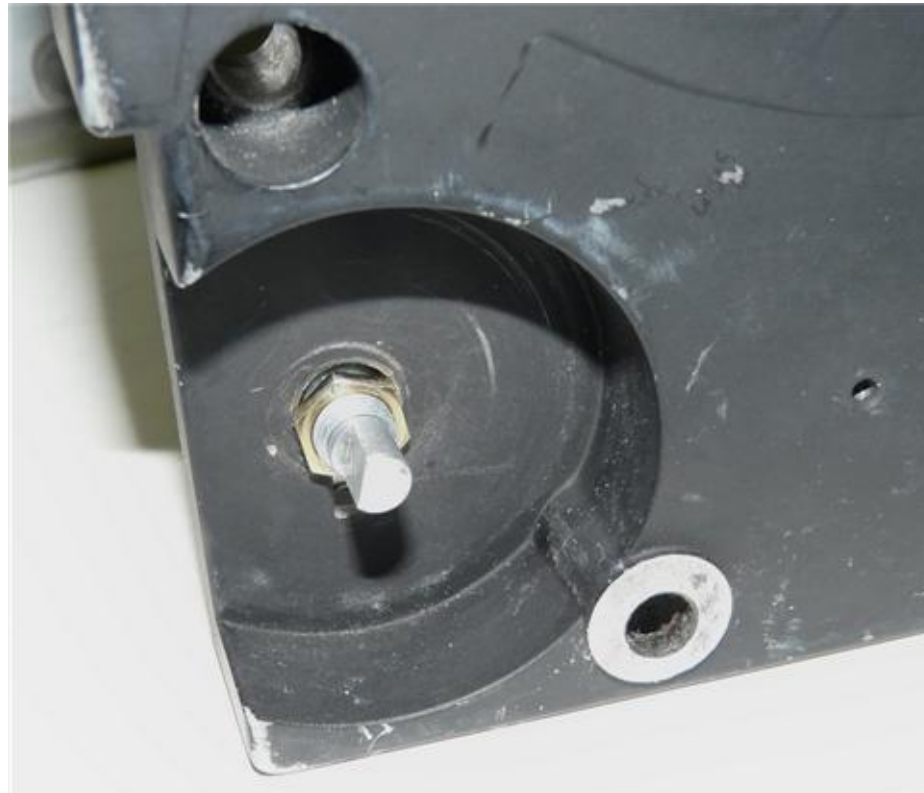
(5) Remove the intensity control wheel.
