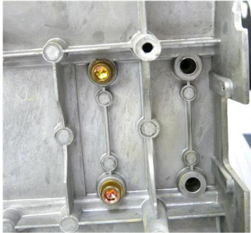
(1) Remove the 2 cap screws closest to the back of the microscope. (the ones holding the neck to the base) Use the 5mm hex key.
