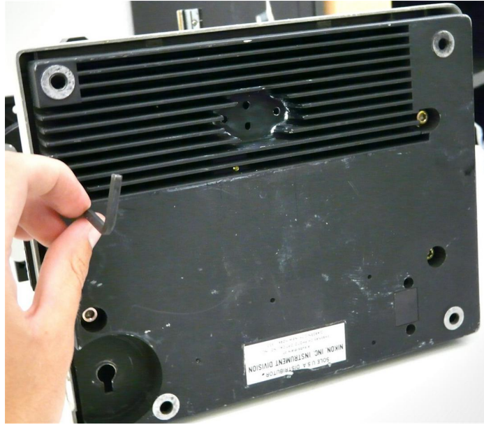
(1) Remove the 4 cap screws with the 4mm hex key.
