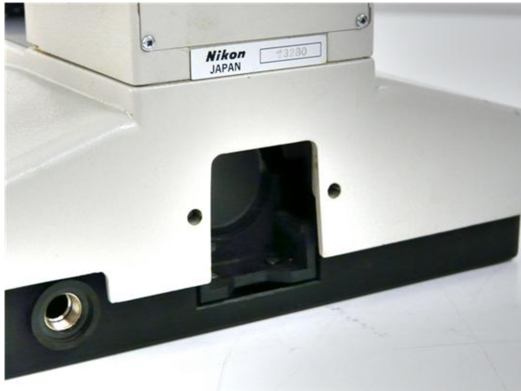
(4) Remove the original lamp housing.
