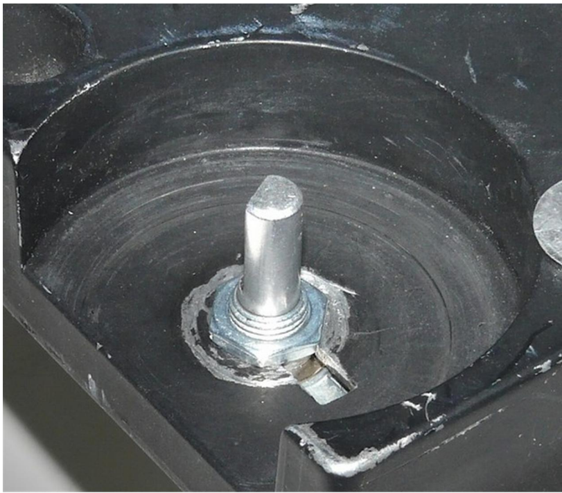
(5) Secure the pot with the included nut. Use an 11mm socket.
