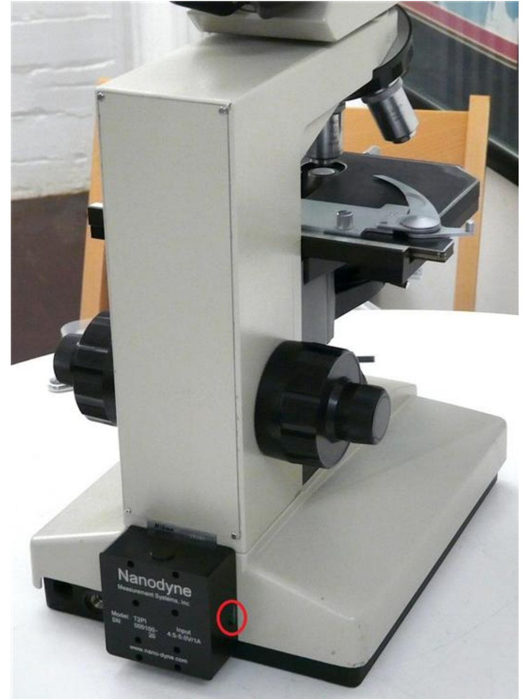
(2) Connect the USB end of the power cord to the power supply and the other end to the illuminator at the red circle. Plug the power supply into an AC outlet and it is ready to use.
