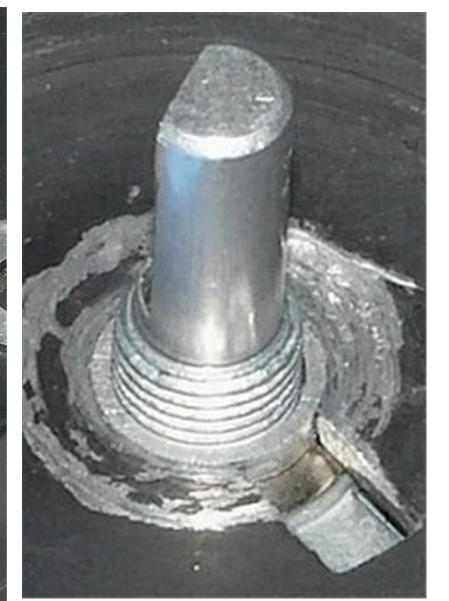
(4) Close up showing the metal centering bushing.
